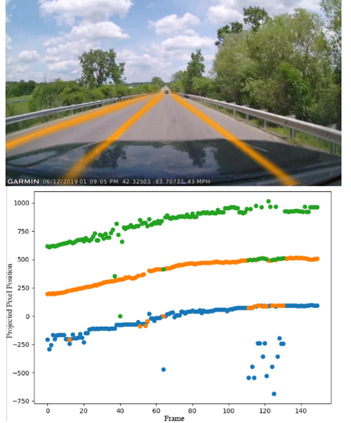
Fig. 4. Graph of the location of each lane (in pixels) in the dashcam against time for a typical lane change. Each color shows the inferred position of a specific lane.
